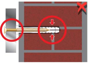
Nail-in anchor does not expand \*Sleeve can't grip inside of hole \*Will pull out - object will fall off wall
