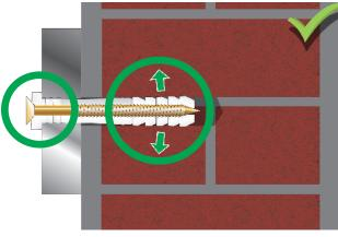
Nail-in anchor expands fully \*Sleeve grips inside of hole \*Object stays on wall
